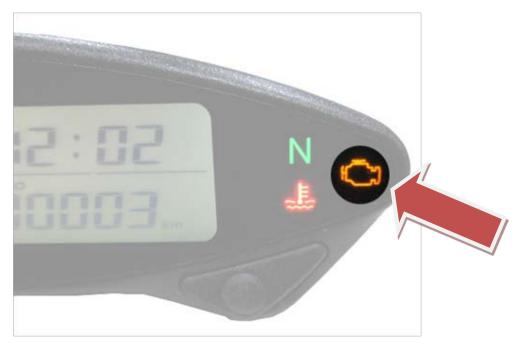
To know what is the fail and how proceed you can check the "On Board Diagnostic (OBD) Manual" that describes step by step how solve the errors show bu OBD tail light
